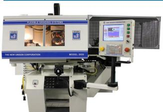
The **Model 2650** Combination Cutting Tool/Burr Grinder shown with optional autoloader is a rigid, but compact, proven version of our Flexible Grinding System™. It features a fully enclosed work area and includes an automatic steadyrest, part location gage and collet for a specific shank size.
